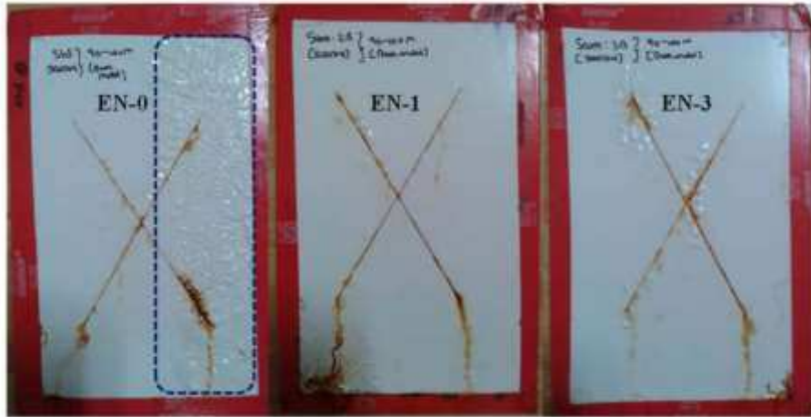
Coated panels after 500 h salt spray chamber [3]
