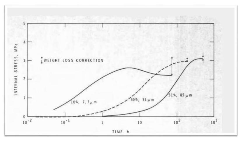
Development of internal stress, showing initial solution concentration (% WIW) and dried coating thickness (pm) (Croll, S. G. Journal of Coatings Technology, Vol. 50, No. 638, March 1978, 33-38)
