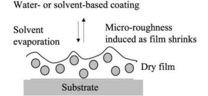
• Fig.2. Matting mechanisms. Typically a liquid precursor system with matting agent is initially applied to a substrate (top). In a conventional water-or solvent-based system, evaporation of this liquid leads to surface roughness and segregations of matting agents near the coating surface (bottom, right). In a UV-curable coating, segregation of matting agents is more difficult as there is not a significant change in the volume of the film during curing (bottom, left).
