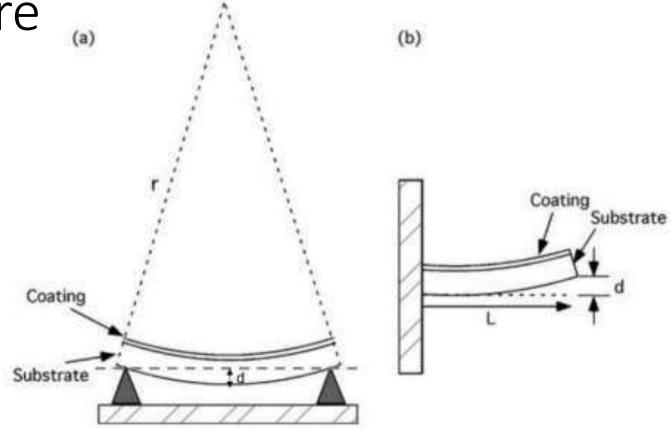
Schematic diagram of set-up for curvature (a) and cantilever deflection (b) method to monitor internal stress in coatings. (Li, Q., 2022, Quantification of internal stress and cracking in ambient temperature curing thermoset coatings. Technical University of Denmark.)
