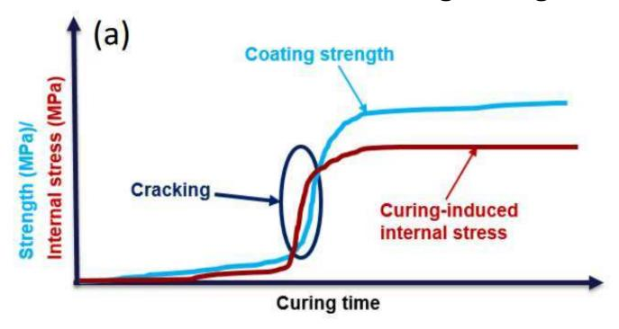
Schematic illustration of the coating strength and the internal stress development during curing. (Li, Q., 2022, Quantification of internal stress and cracking in ambient temperature curing thermoset coatings. Technical University of Denmark.)
