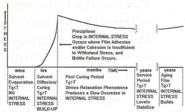
Development of internal stress in a solventborne paint with no polymerization (Clive Hare Aircraft Paint Stripping News II Summer, 1997)
