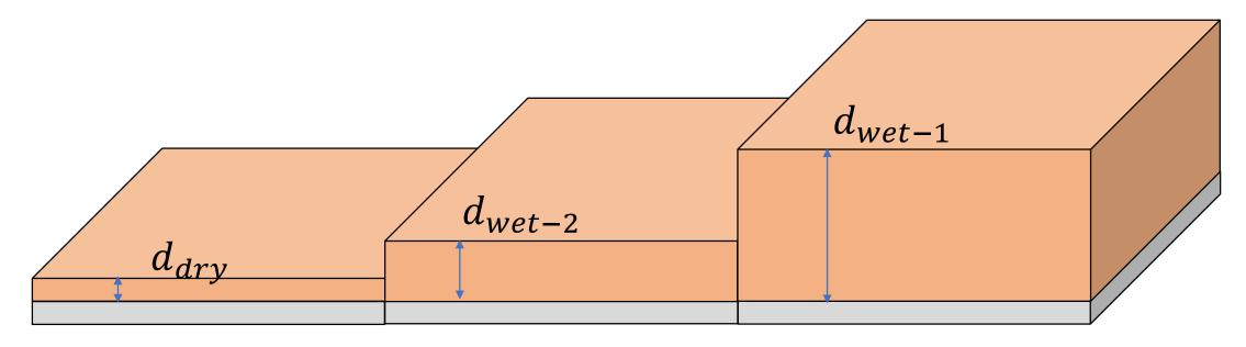
Shrinkage due to loss of volatiles and polymerization. Notice the volume change involves only one dimension.
