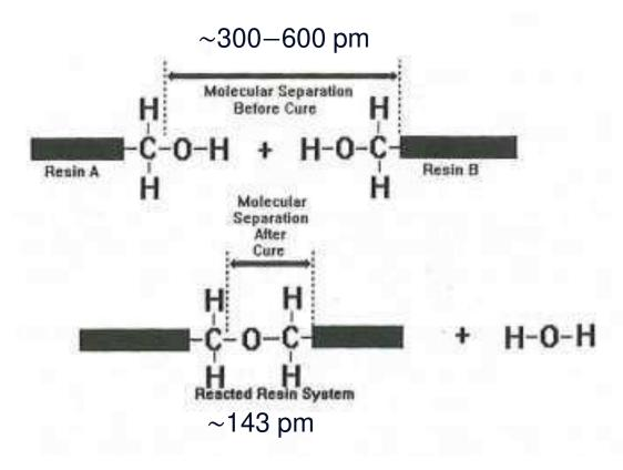
Shrinkage on polymerization as a source of internal stress (Clive Hare Aircraft Paint Stripping News II Summer, 1997)
