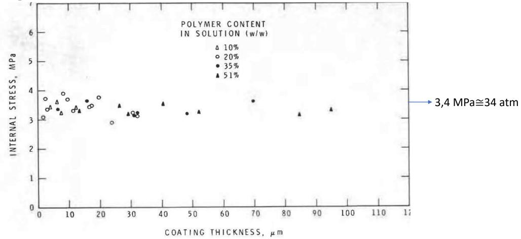
Development of internal stress, showing initial solution concentration (% WIW) and dried coating thickness (pm) (Croll, S. G. Journal of Coatings Technology, Vol. 50, No. 638, March 1978, 33-38)
