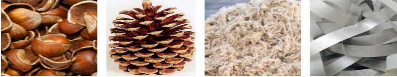
Fig. 1. Filler materials used in specimen production (a-hazelnut shells, b-pinecone, c-waste sheep wool, d -wastepaper).
