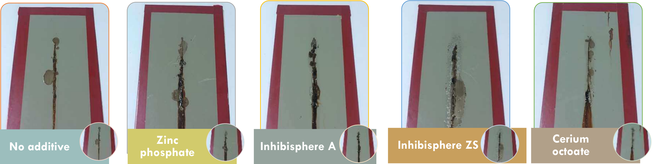
Figure 3: Panel's photographs after 500 hours corrosion test
